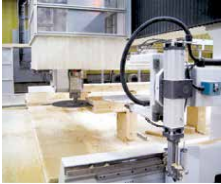
Modern Computer Numerically Controlled (CNC) connections provide the ability to fabricate joints with precision. This is especially useful when fabricating joints on large members with complex shapes.
