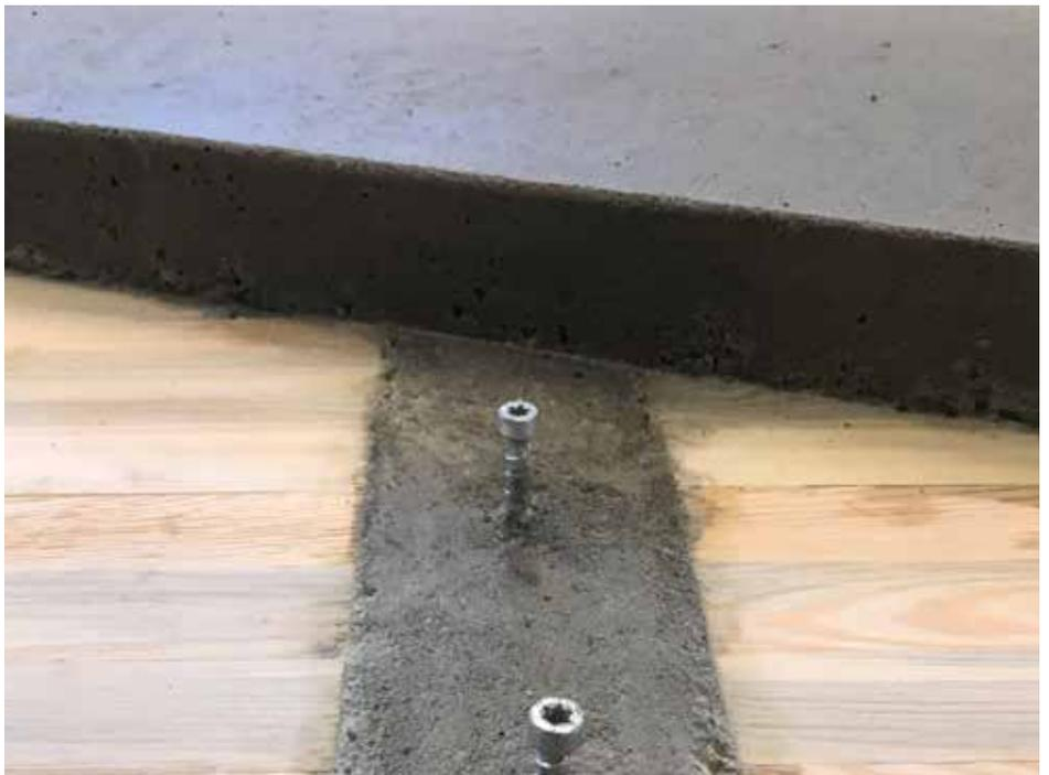
Most mass timber panels can be made into a wood-concrete composite by applying a concrete topping in such a way that the two materials act as one. Product sample courtesy of StructureCraft
